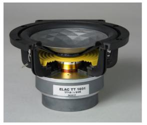
• The design of the woofer is based on the renowned ELAC aluminium sandwich technology. The crystallike surface of the new aluminium membrane catches both the eye & the ear. Distortions are significantly reduced by the angled crystalline surface structure. In addition, by using this pressformed structure, the membrane is more rigid, which not only prevents partial vibrations in the crossover
